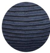
Structured knit fabric knitted along side out of spark nylon yarn, forms a circle when put down.
