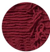
This series achieves a variety of expressions through knitting only one of the layers of a double-knit wool fabric, with water-soluble thread.
